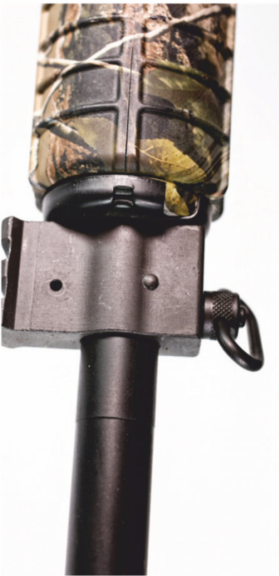
The gas block is fixed and has a rail on top in case you want to mount back-up iron sights. Depending on how hard you are on optics, that might not be a bad idea.
