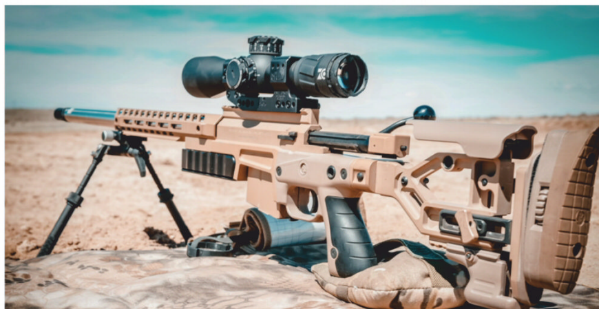
Accuracy International's AXSA is a short-action, multi-caliber rifle. Currently chambered in 6.5CM, it was originally conceived as a .308. Barrel and caliber changes take under two minutes to accomplish.
